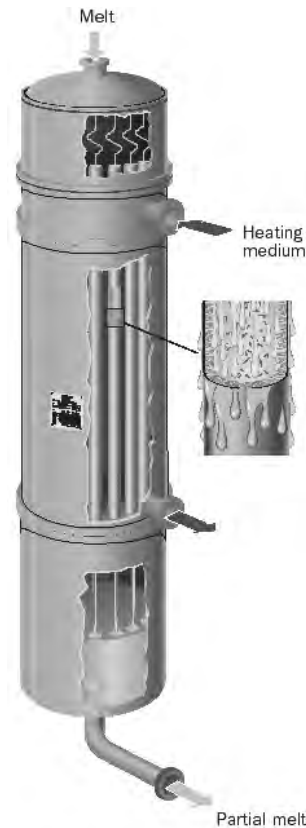
Figure A.2: Falling film crystallization: the melt flows down on the inside surface of the tubes, whereas the medium used for cooling is distributed to wet the external surface of the tubes [151].
