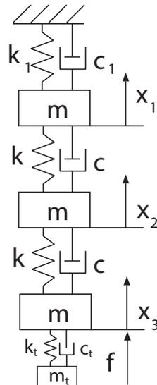
Figure 2 – 3-DOFs system equipped with a Tuned Mass Damper (TMD)
