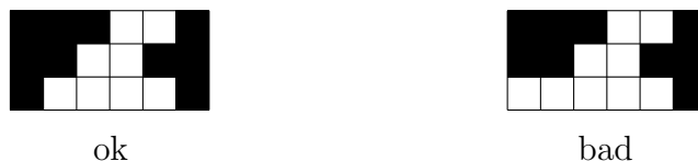
Figure 5: When c = 2 , the left segment respects the interleaf distance constraint while the right segment does not because the first left leaf is in position 4 and the last is in position 1.
