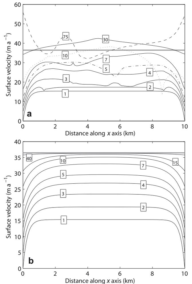
**Fig. 3.** Successive true Picard approximations of the surface velocity for an infinite parallel-sided slab of isothermal ice on a sloping bed (see text for details). Results are given for (a) a finite-difference implementation (Pattyn, 2002) and (b) a finite-element implementation. Numbers on the curves correspond to iteration numbers. The thick grey line gives the exact solution.
