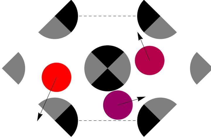
**Figure 2.** Two-dimensional lattice billiard with rhombic tiling. The walls of the left and right cells (in grey) are thermalized to unit temperatures. The horizontal lines in the middle cell indicate periodic boundary conditions. The particle in the middle cell is subjected to the usual rules of elastic collisions when it collides with the fixed discs at the four corners of the cell, or with the moving particles in the neighbouring cells.
